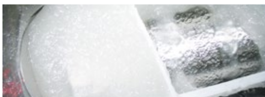
Abb. 4: Erzeugung von PCS mittels Scraped Surface Slurry Generator Fig. 4: PCS generation via Scraped Surface Slurry Generator
