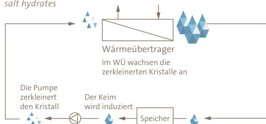
Fig. 3: Procedure for generation of PCS using slowly crystallising salt hydrates
