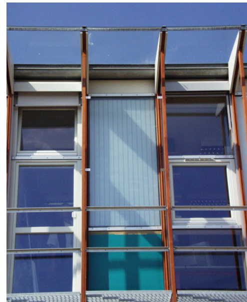
Fig. 2: Test façade for thermal characterization of windows and façade systems under real conditions
